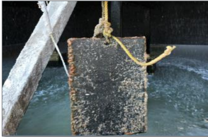
4 months after immersing fouling plate ( Before Chlorine Dioxide Trial )
