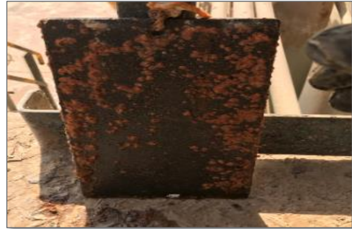
4 months after immersing fouling plate ( Before Chlorine Dioxide Trial )
