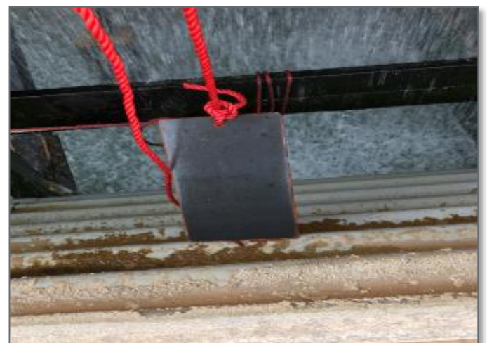
14 months after immersing fouling plate ( After Chlorine Dioxide Trial )
